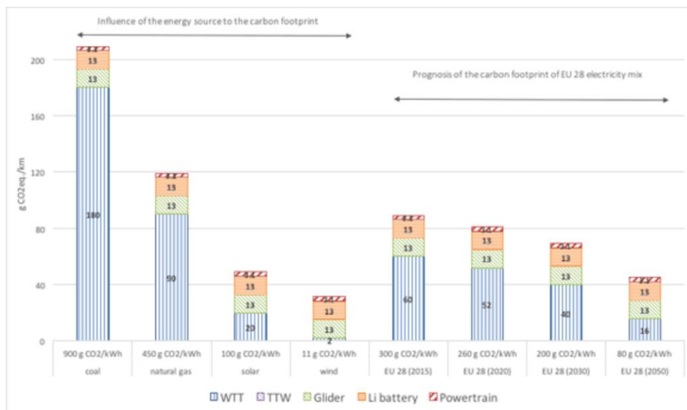
Figur 5. GHG emissions of electric vehicles depending on the energy sources and the prognosis of the reduction in carbon intensity.
